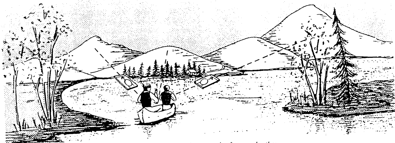
When resectioning, use landmarks that are at about 45-to 90-degree angles from each other.
