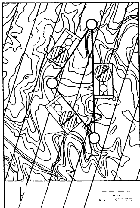
Map with magnetic lines drawn. This method avoids adding and subtracting declination.
